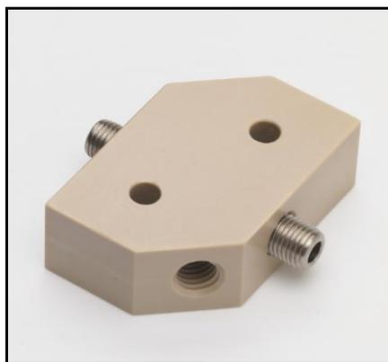
The line of fiber optic **SMA Z-Cells** is the top choice for many absorbance measurements. SMA-Z-Cell path lengths are available between 2.5mm - 100mm and can be made in PEEK, Plexiglas, Stainless Steel, Teflon, and Ultem. The cells contain fused silica windows and are compatible with standard SMA-905 terminated fiber optic cables.
