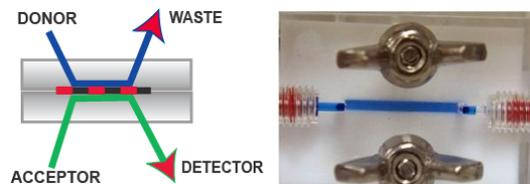
Flow scheme of gas diffusion unit and its photo shown from acceptor side. Unit dimensions are 4cmW, 2cmD and 3cm.
