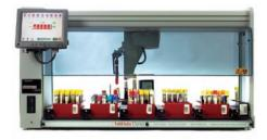
The PathFinder 350S Sorter is an open, fully automated, stand-alone system that is designed to manage pre- and post-analytical sorting, storing and tracking in a pathology laboratory.
